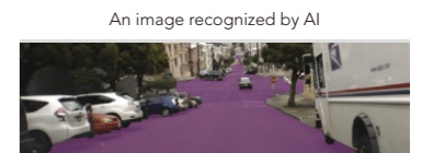
An image recognized by AI Can focus solely on the road surface even in complex road environments (Color-codes the recognized road surface on a pixel-by-pixel basis)
